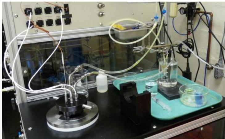
*Figure 1: Set-up of previous dissolution experiments using the Autolab 1000 where the fluid composition is constantly monitored.*
