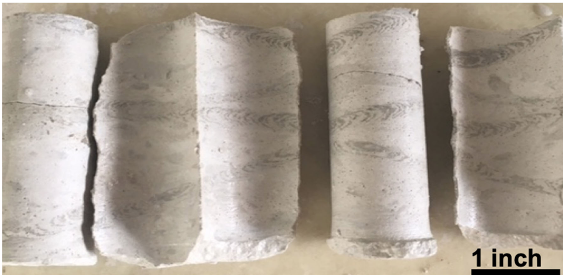
Figure 1: One inch plugs of fine-grained wackestone with tiers of Zoophycos that is one of the typical ichnogenera for carbonate contourite drifts.
