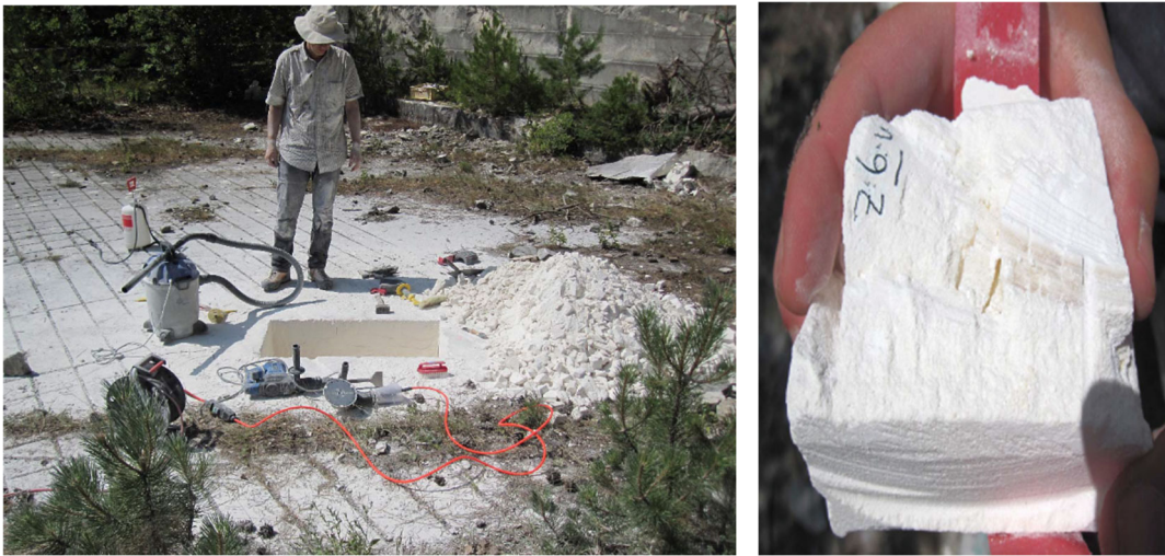
Figure 2: Left: The excavated hole on the quarry floor to one of the shallowest of dots imaged on a GPR stratal slice revealed that the dot signature was produced by a rudist of about 10 cm length (right).
