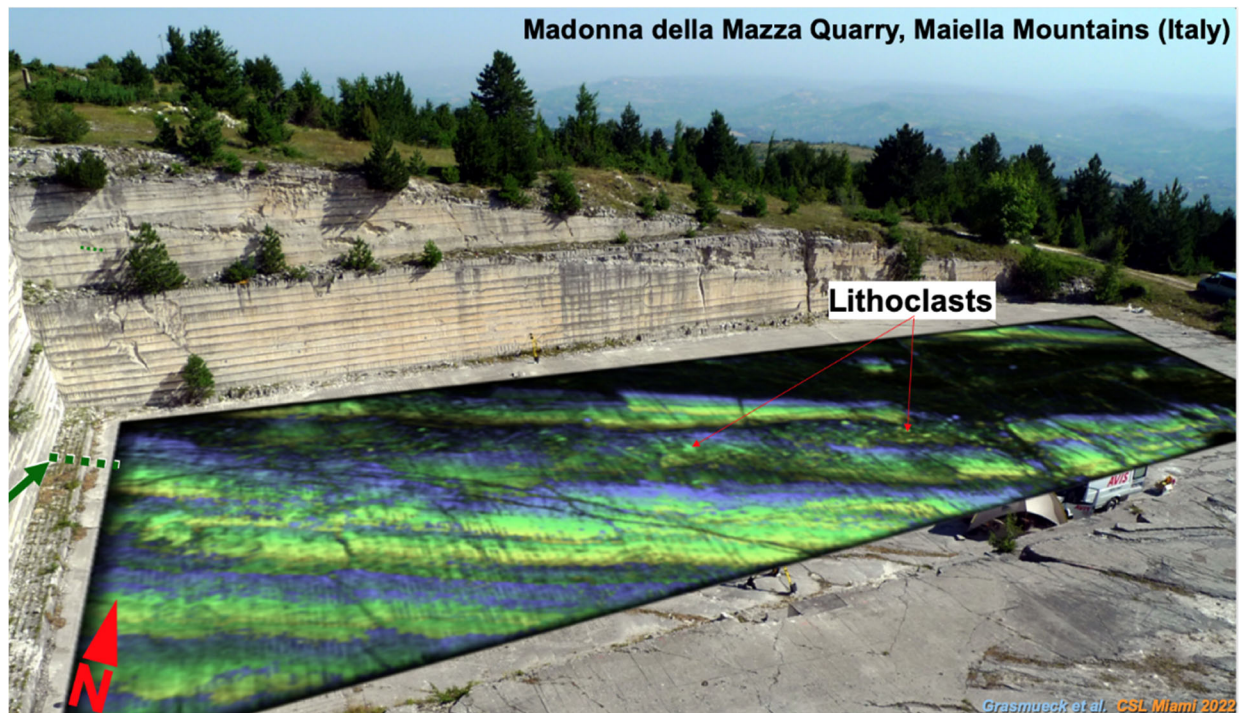
Figure 1: Madonna della Mazza quarry with stratal slice of dipping beds using the pond view technology applied in the high-resolution 3D GPR cube that was acquired in the quarry.
