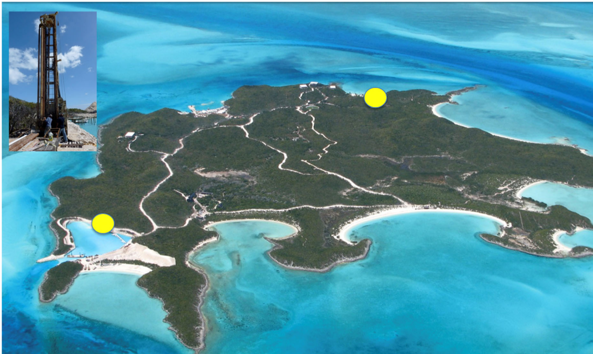
Figure 1: Bell Island with the location of the two disposal wells that were drilled down to 183 m (600') thereby providing the deepest record of the Exumas windward margin. Inset: Drill rig used to drill the disposal wells.
