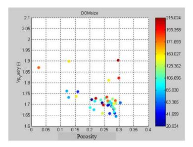
Figure 1: Cross plot of porosity and Vp/Vs ratio for a sample set of dry measurements from a Middle Eastern limestone reservoir. Superimposed is the digital image analysis parameter Dominant Poresize (in microns). No clear relationship is visible between pores structure data and Vp/Vs ratio. Vp/Vs ratio shows a negative correlation with increasing porosity, indicating that Vp/Vs ratio is non-constant with porosity.
