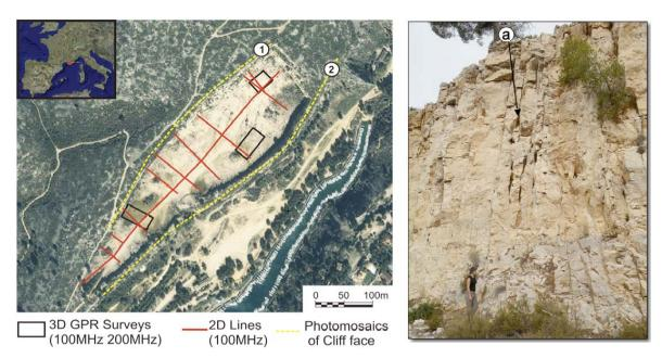
Figure 1: Left: Map of Cassis Quarry: The quarry is over 500 m long and approximately 100 m wide, allowing for the examination of production scale lateral variability of the fracture network. The location of the 2D and 3D GPR data acquired in 2008 is shown. LIDAR scans of the cliff faces adjacent to the Quarry floor will be acquired in 2009. Right: Near vertical fractures in the quarry wall. Marker a shows how some of the fractures are solution enhanced.
