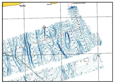
Figure 2. Analog bathymetric data from the proposed study area south of Grand Bahama Island (yellow at top of figure). The channelized slope is easily visible in these data.
