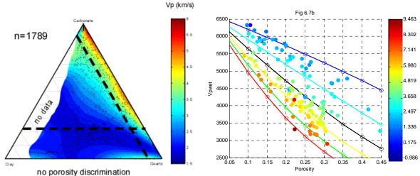
Figure 1: Example ternary diagram showing the relationships between P-wave velocity and textural and mineralogical composition (from Kenter et al. 2007) (left); Cross plot of porosity vs. P-wave velocity with the gammaK parameter from Sun's Extended Biot Theory superimposed. The gammaK parameter captures the frame flexibility at a given porosity and provides a mean to relate the pore structure of carbonate rocks to acoustic velocity variations (Weger et al. In press).
