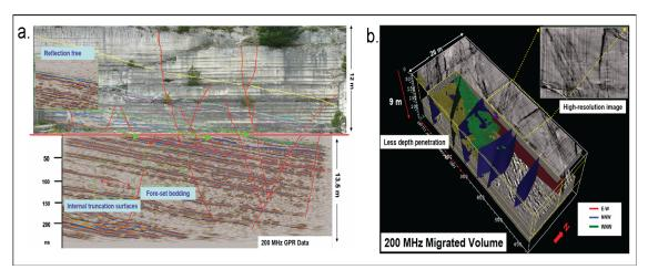
Figure 2: a). Quarry wall with fractures and bedding surface traced into the subsurface in the 100Mhz GPR volume. b). 200 MHz migrated volume with stratigraphic and fracture interpretations.
