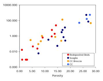
Figure 1: Porosity versus permeability of megabreccias and turbidites (red dots) and the corresponding background sediment (Scaglia, dark blue dots). Breccias rich in rudist debris (Calcare Cristallini, orange dots) have generally less porosity and permeability than the coarse-grained rudist grainstone (Calcare Cristallini, CC, light blue dots).
