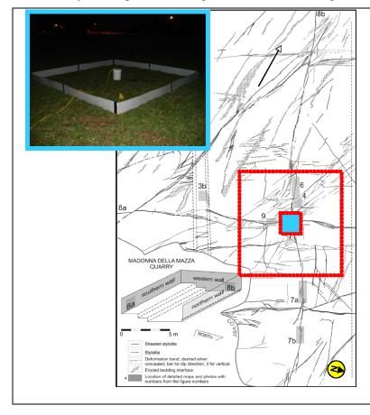
Figure 3: Location of the proposed ponded infiltration experiment on the Tondi et al (2006) map (blue square). The larger stippled square is the footprint of the repeat 3D GPR surveys. To avoid GPR antenna surface coupling artefacts we will construct a temporary pond using white plastic sheets (see inset). After all water has infiltrated, the pond walls are removed and the first post-infiltration GPR survey can be recorded.
