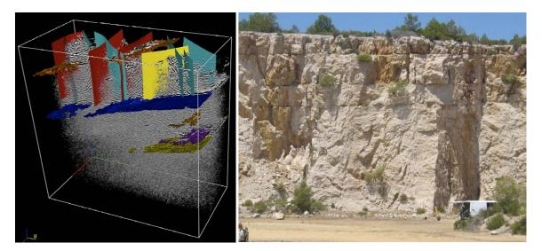
Figure 2: Left: GPR volume (values of minimum amplitude are removed) with stratigraphic and fracture interpretation. The blue horizon acts a mechanical unit boundary against which the large fractures terminate. Right: A major fault offsetting the quarry wall is one of the green faults interpreted in the GPR data. This fault like most fractures strike N080° and are sub-vertical.
