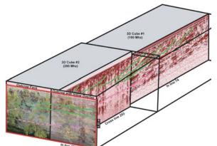
This figure shows an outcrop photo and two ground penetrating radar cubes.
