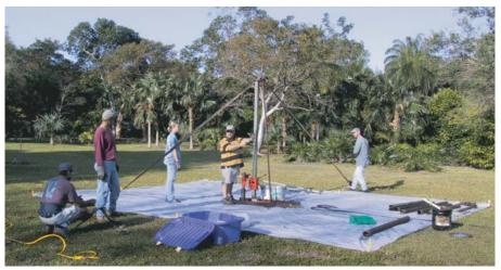
Drilling team working to get a core from the Miami Oolite that would be used for ground-truthing the GPR data and laboratory measurements.
